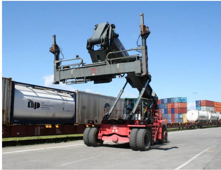
Figure 4: Reach stacker usable for lifting and transporting empty Transport Unit (Source: UWB)
