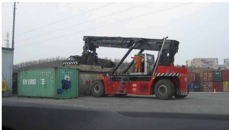
Figure 5: Empty TU manipulation using top-lift spreader equipment (Source: UWB)
