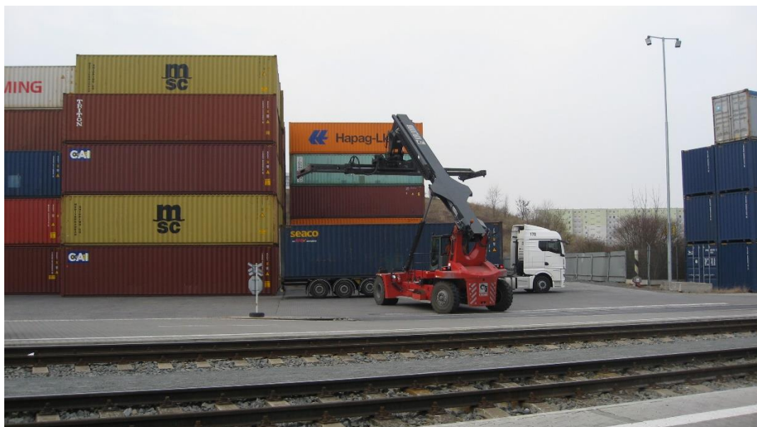
Figure 6: Cargo container handling via Reach stacker (Source: UWB)
