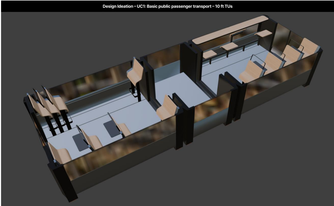
Figure 8: Mixed TU interior layout for UC1 (© moodley)
