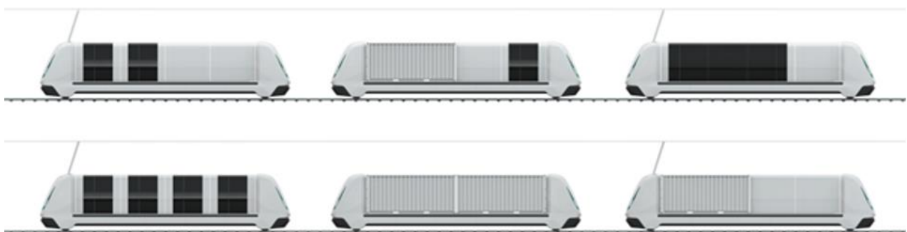
Figure 6. Possible configuration (TU type A and 20' containers) on rail carrier
