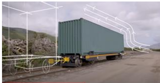
Figure 2: Container being transported by Parallel bogies, rendering of interaction with additional bogies and aerodynamics. Source: video credit, @Parallel Systems, 2023
