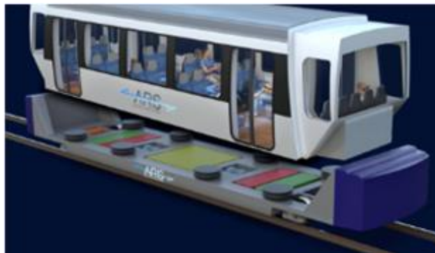
Figure 3: Decoupling of chassis and passenger compartment design. Source: @ifs, Benno Schiefer, RWTH Aachen University, 2022
