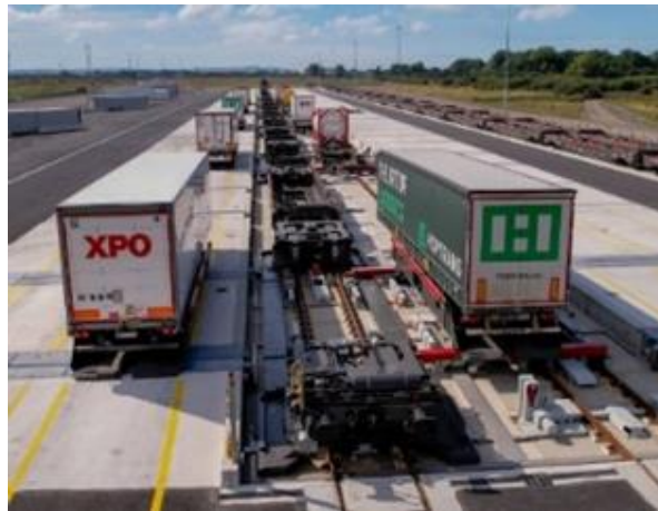
Figure 25: Several semi-trailers ready for the simultaneous transshipment. Source: ©CargoBeamer AG, 2021
