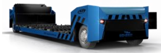
Figure 18: Rendering of Gaussin’s Autonomous Airport Transporter. Source: Gaussin Group, Public Domain, 2023
