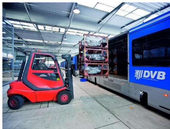
Figure 46: Grid-boxes being loaded by a forklift onto a Dresden CarGoTram. Source: @Sachsen Fernsehen, 2017
