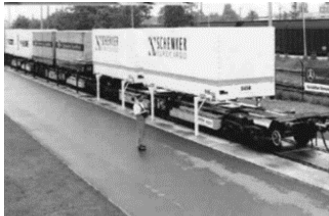
Figure 31: Kombilifter swap body with extended legs positioned on the railway siding of the Mercedes-Benz factory in Stuttgart. Source: Mercedes-Benz, Public Domain, 1995
