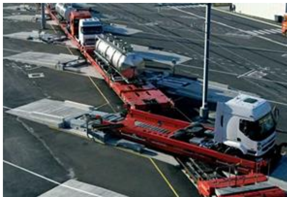
Figure 26: Pivot basket in diagonal position ready to be aligned with the train formation. Source: ©Lohr Industrie S.A., 2003
