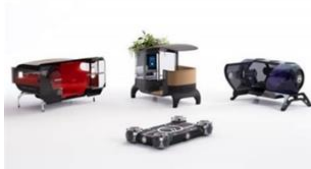
Figure 13: Citroën Skate round-wheel carrier and its three transport units Sofitel En Voyage, Citroën X JCDcaux, and Citroën X Accor. Source: ©Citroën, 2023
