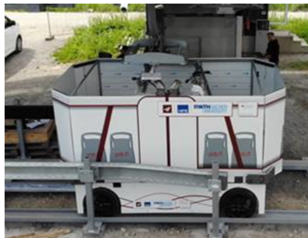
Figure 22: Screenshot of the transhipment test of the transport unit from the road carrier directly being coupled to the ropeway grip. Source: video credit of the RWTH Aachen University, 2021
