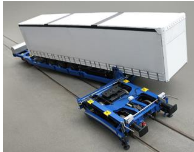
Figure 27: Rendering of the swivelling structure of Trailer Rail, former Kockums Megaswing Duo. Source: SGKV Intermodal Info, Public Domain, 2010
