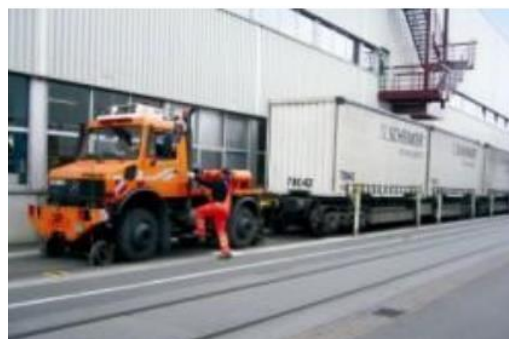
Figure 35: Kombilifter swap body with extended legs positioned on the railway siding of the Mercedes-Benz factory in Stuttgart. Source: Mercedes-Benz, Public Domain, 1995
