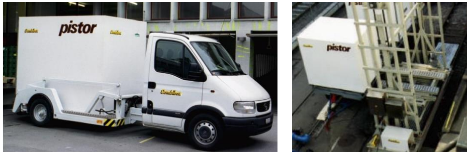
Figure 37: Combibox carried by an adapted van and being transhipped on to a freight wagon. Source: Tiefbauamt der Stadt Zürich, Public Domain, 2002
