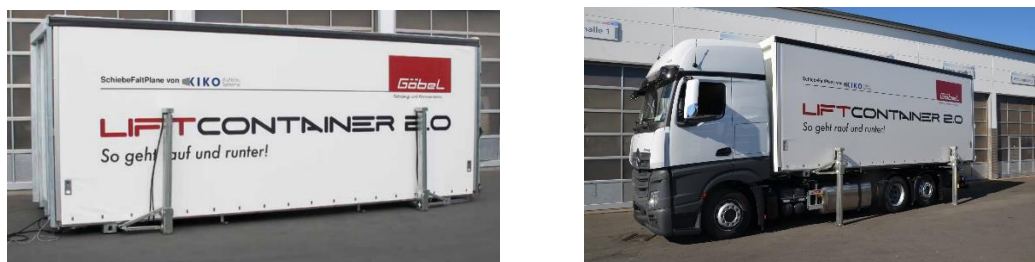
Figure 38: Liftcontainer with folded legs and, secondly, with extended legs prepared to be docked on to a truck. Source: @Liftcontainer.de, 2020
