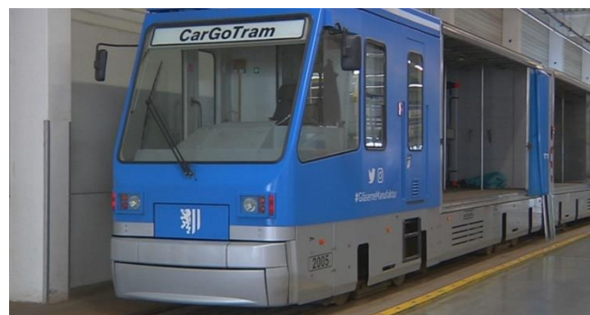
Figure 51: Dresdner CarGoTram only cargo raised floor cargo-tram vehicle concept with open curtain side for the loading process. Source: ©Sachsen Fernsehen, 2017
