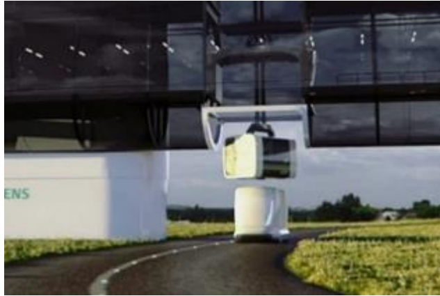
Figure 1: Transport unit being conveyed from Road mode to Ropeway mode. Source: video credit of moodley / Siemens Mobility, Public Domain, 2022
