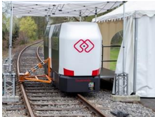
Figure 59: Monocab being tested with a provisional support. Source: @Monocab OWL, 2023
