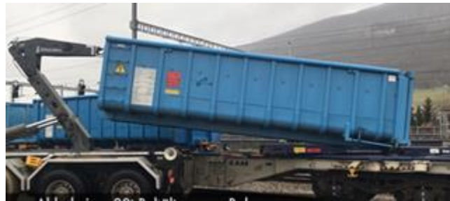
Figure 33: Roller container with hook during transshipment of a 30 t container. Source: video credit, ©ACTS Abroll-Container-Transport-Service AG, 2019
