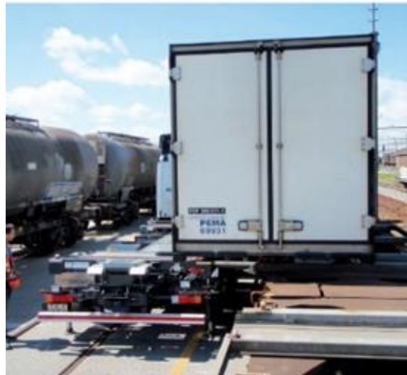
Figure 24: Horizontal rail-road handling of a semi-trailer with the ContainerMover of InnovaTrain. Source: InnovaTrain, Public Domain, 2010
