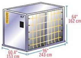
Figure 49: Air freight, Unit Load Device (Types & Dimensions), Source: ©TVM Global, 2015
