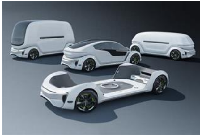
Figure 16: Visualisation of the conceptual Tesla pod system with a carrier and the three envisioned transport units, published by Yanko Design. Source: ©Fábio Martins, 2019
