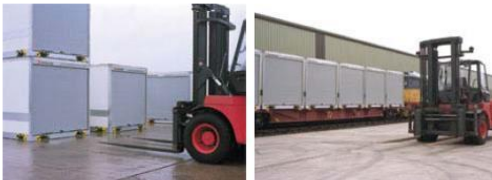
Figure 34: Minimodal small-sized containers being handled by a standard forklift. Source: Rail Freight Limited, Public Domain, 2002
