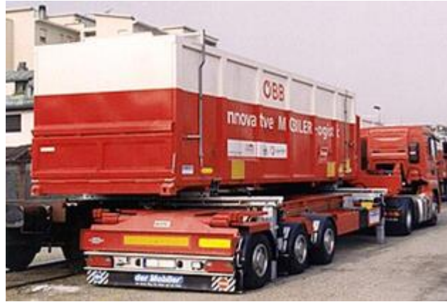
Figure 23: Horizontal handling of a Mobiler container from a truck to a wagon in parallel position. Source: Rail Cargo Group, ÖBB, Public Domain, 1995
