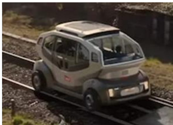
Figure 58: Visualisation of the Flexy two-road vehicle concept driving on the railway close to a level crossing. Source: ©SNCF, 2021
