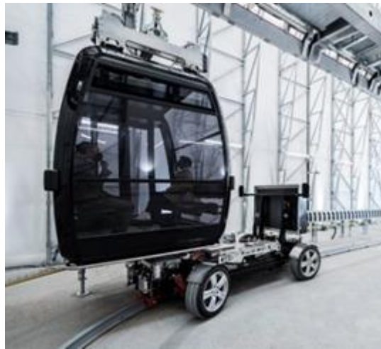
Figure 8: Docking of ropeway cabin onto road carrier. Source: ©LEITNER AG, 2023
