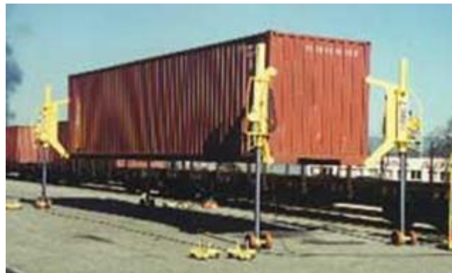
Figure 32: Container supported by the Roll Hydro hydraulic jacks. Source: Construction News, Public Domain, 1994
