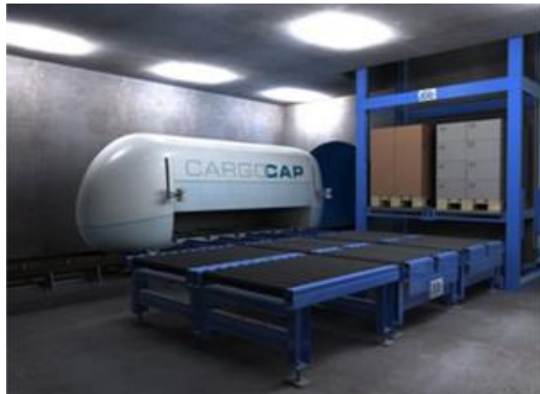
Figure 53: Visualisation of the CargoCap transport unit at the freight loading area. Source: ©CargoCap GmbH, 2017
