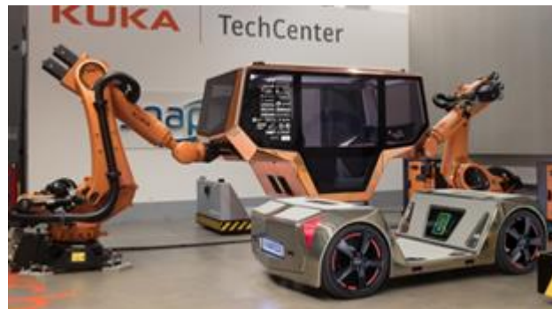
Figure 21: Transport unit of the Rinspeed MicroSnap being transhipped by two KUKA robot arms. Source: ©Rinspeed AG, 2019
