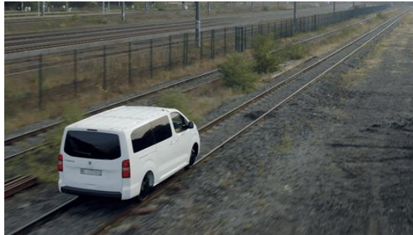
Figure 57: Adapted road vehicle of the Flexmove project during tests on railway track. Source: ©AKKA, 2022
