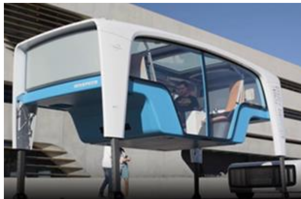
Figure 20: Transport unit of the Rinspeed Snap with its supporting legs extended. Source: video credit, ©Rinspeed AG, 2018
