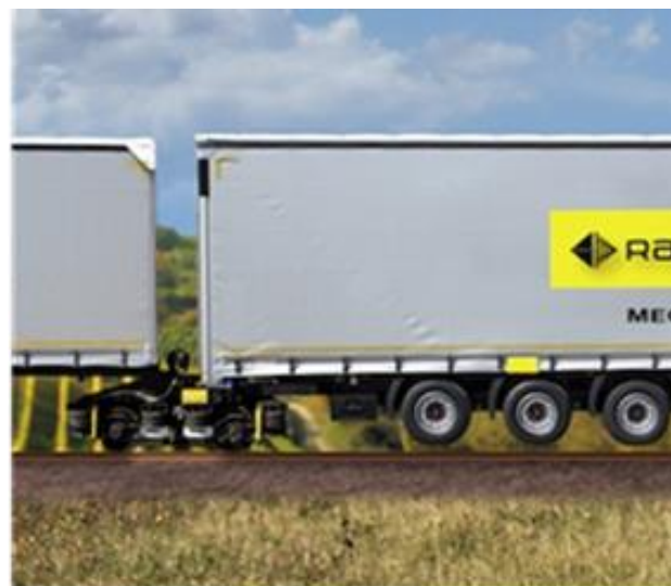
Figure 28: Detail of two semi-trailers coupled to the RailRunner® bogie. Source: RailRunner® North America, Public Domain, 2006
